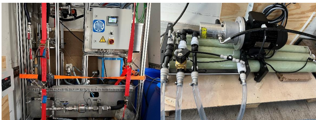
Figure 6: The setup of the ceramic filtration system (on the left) and the reverse osmosis system (on the right).
