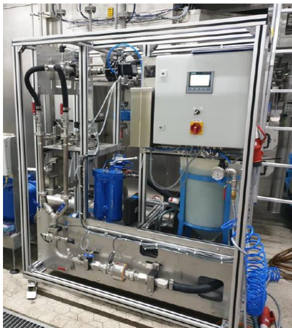
Figure 3: Picture and simplified flow chart of the mobile membrane test plant (Mikro-Mia 2.0)
