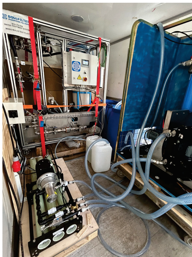
Figure 10: On site setup (in truck); ceramic filtration (top left), reverse osmosis (front left).
