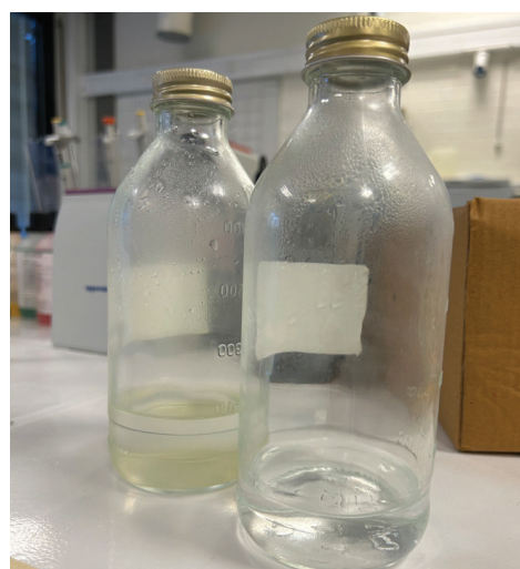
Figure 13: MD feedwater (left) and permeate (right)
