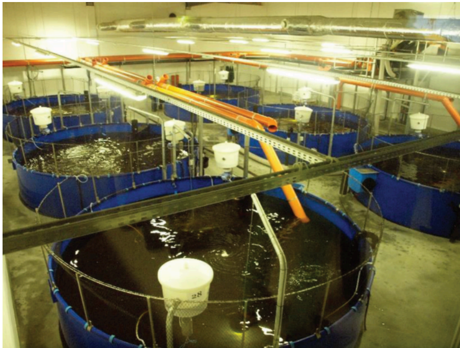
Figure 110. Salmon breeding tanks (5m diameter) – post-smolt cycle phase on the Jurassic Salmon farm. Picture of the author.
