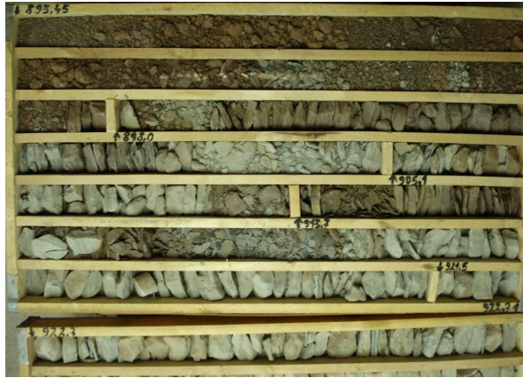
Figure 49. Friable sandstone (Oldred Sandstone), borehole Palanga-138a. Gray and old-red colours are documented in the well. Fine sandstones are cemented by dolomite and an admixture of clay minerals.
