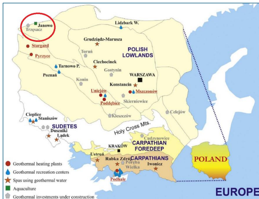
Figure 106. Geothermal energy provinces and installations in Poland
