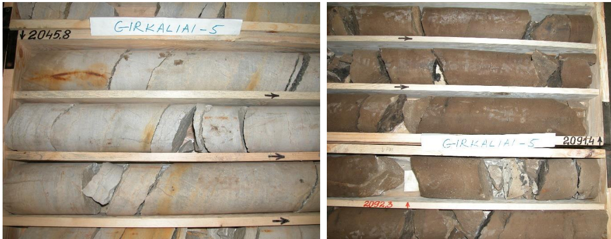
Figure 44. 1 – Strongly quartz cemented sandstones, oil production borehole Girkaliai-5 (Giruliai Fm.); 2 – moderately cemented sandstone stained with oil, borehole Girkaliai-5 (Pajūris Fm). 30° deviated well. The Vydmantai boreholes are located outside the oil field contour.
